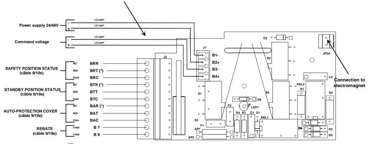
(\*) :Active contacts "unlocked lock" and "Closed cover"
